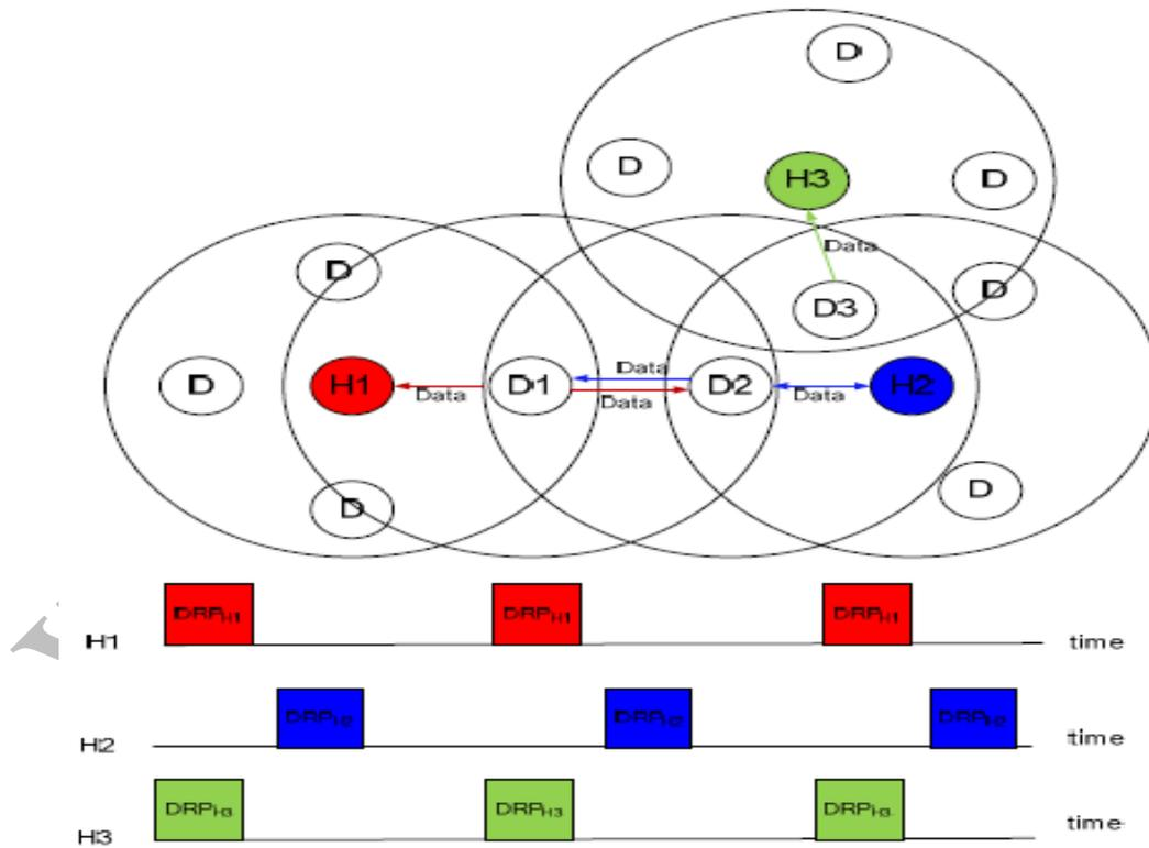
**Figure 2.8. Interference-free data transmission during each DRPH1 and DRPH3.**
