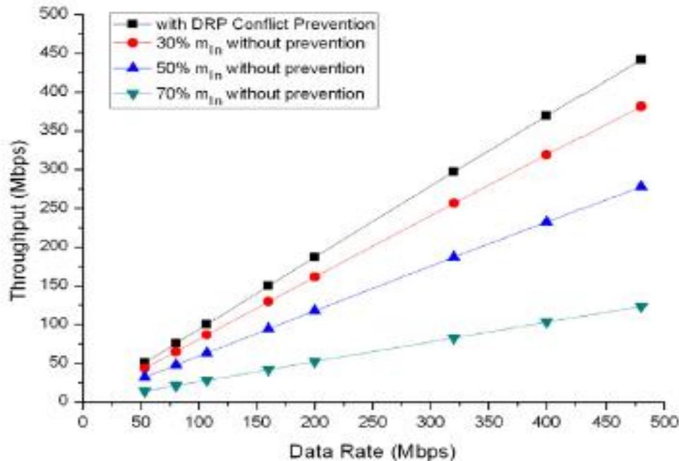
**Figure 4.1 Throughput of a WUSB device according to each UWB PHY data rate.**
