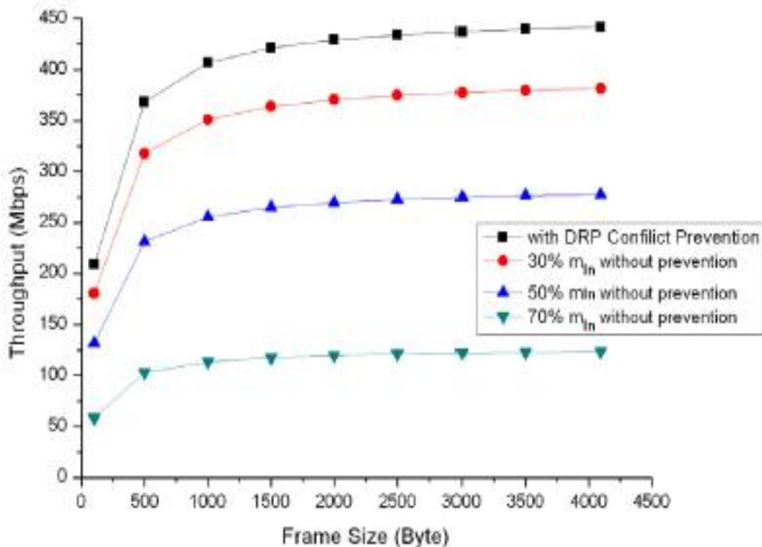
**Figure 4.2 Throughput of a WUSB device according to each frame size.**
