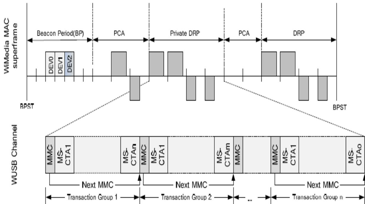
**Figure.2.1** The example of the data exchange between WUSB devices through WiMedia D-MAC.
